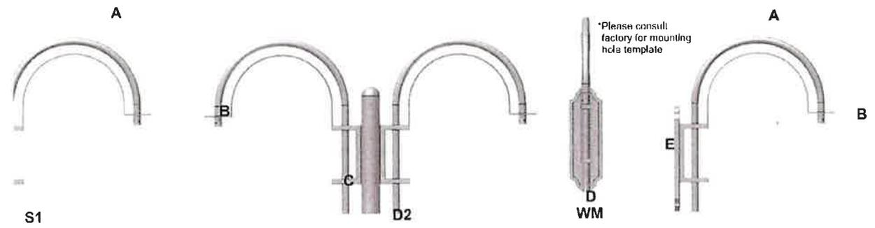
The VA102-L and VA102-M crook arm dimensions are for standard size 2 or size 3 Architectural luminaires only. VA102-S is standard for smaller, size 1 luminaires. Center section of arm will match pole design (i.e. fluted pole = fluted center arm section).
